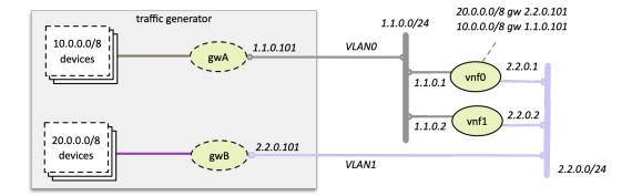
The main advantage of this mode is that only 2 network segments are needed to support an arbitrary number of chains.
