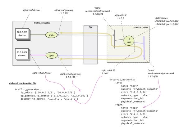
L3 routing must be enabled in the VNF and configured to:
