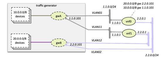
The advantage of this mode is that the configuration of the VNFs can be made identical (same gateway IP addresses, same static routes). However this mode requires 2 network segments per chain.
